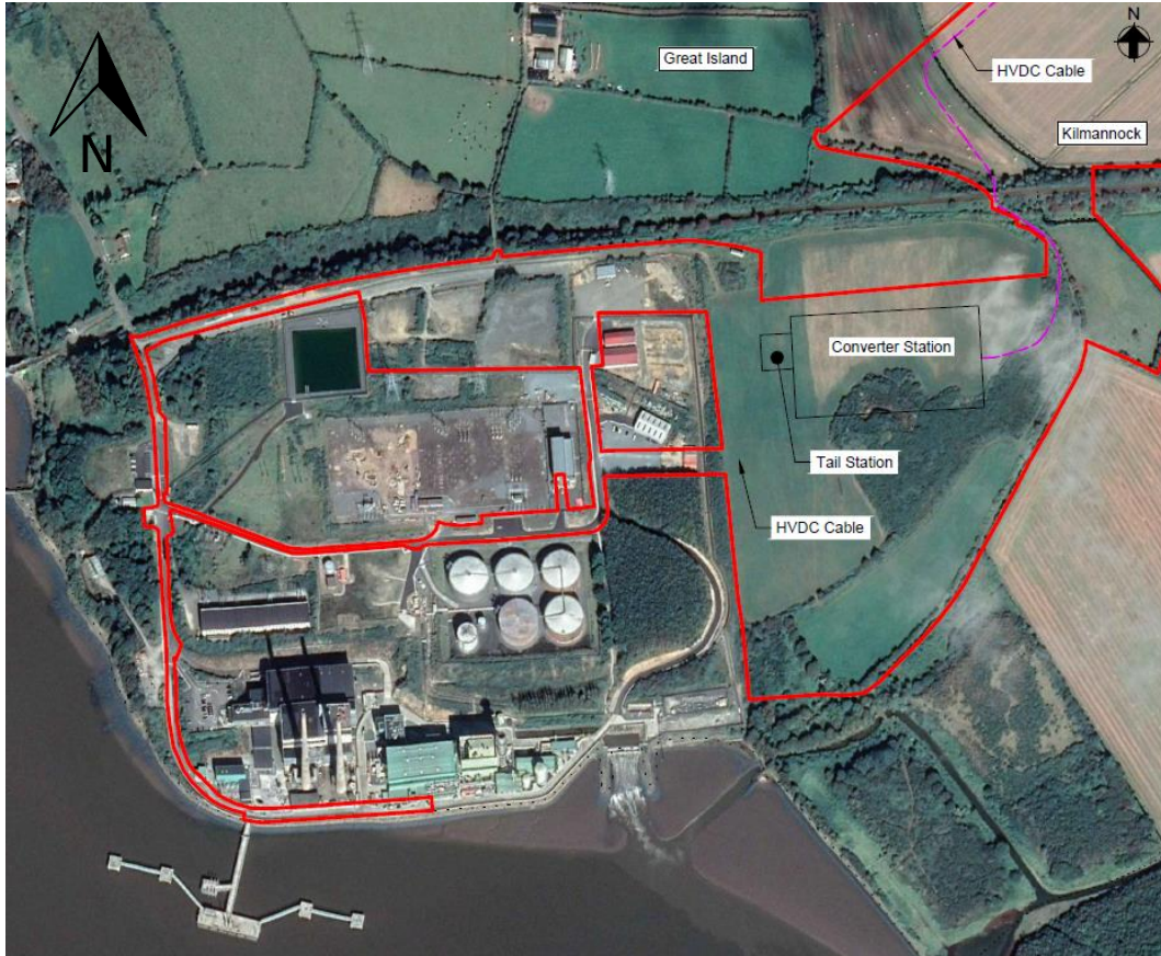
Figure 10.15 Proposed Cable Route and Converter station and tail station at Great Island (mapping source: Bing Maps © Microsoft 2020 | not to scale)
